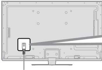
**Insert the power cord plug (included) firmly into place.**
