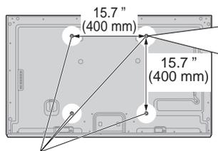
Holes for wall-hanging bracket installation
