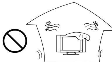
**21. Heat sources** --- Do not install near any heat sources such as radiators, heat registers, stoves, or other apparatus (including amplifiers) that produce heat.
