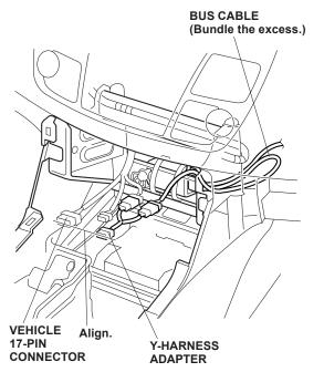
19. Bundle the excess bus cable, and wrap one wire tie around the bus cable.
