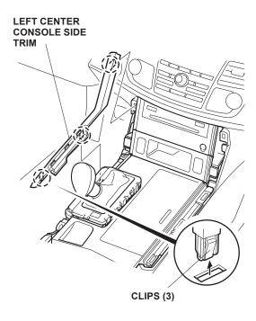
8. Open the center console, then remove the beverage holder (six clips).
