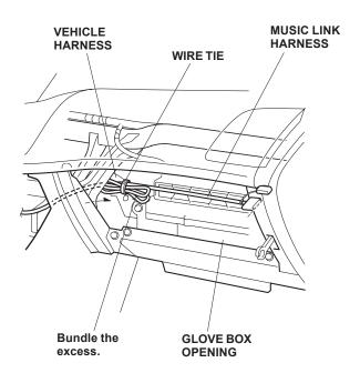
16. Get the Y-harness adapter cable. Connect one end of the bus cable 14-pin connector to the Music Link, and the other vehicle 14-pin connector to the Y-harness adapter connector.
