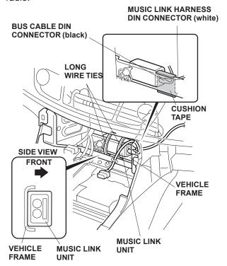
15. Align the Music Link connector with the right side of the glove box opening. Bundle up the Music Link harness and secure it to the vehicle harness with one wire tie.
