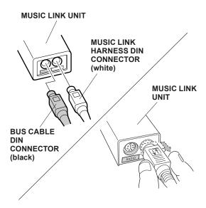
14. Apply a cushion tape around the bus cable DIN connector (black) and Music Link harness DIN connector (white). Secure the Music Link unit to the front side of the vehicle frame using two long wire ties. If the Music Link unit is not in front of the frame there will not be clearance for the radio.
