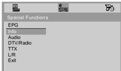
Press the M button to bring forth the program information and hold it on for 1.5s to exit from this interface.
