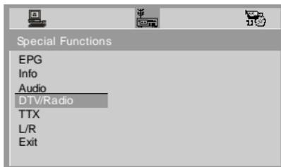
Press the M button to switch the channel between TV and Radio at this status.
