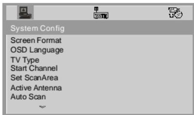
2. Press ◀ or ▶ buttons for to highlight the icon of the desired page, then press the ▲ or ▼ buttons to activate that page.
