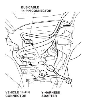
22. Make the length of the Y-harness adapter 14-pin connector the same length as the vehicle connectors. Bundle up the excess length of bus cable, and secure it to the vehicle harness with three wire ties.
