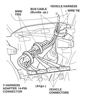
23. Plug the vehicle connectors and the Y-harness adapter 14-pin connector to the audio unit, and reinstall the audio unit.
