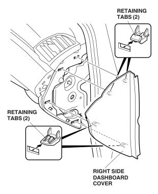
6. Remove the right dashboard trim (one self-tapping screw, ten clips, and three retaining tabs).
