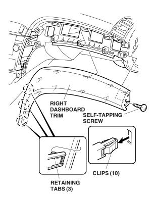
7. Using a flat-tip screwdriver and a shop towel, remove the driver's side center trim (five clips and three retaining tabs).
