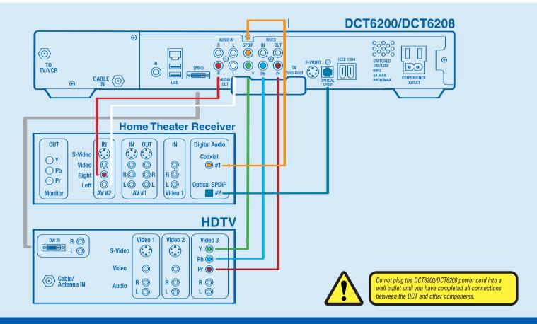
To take full advantage of the DCT6200/DCT6208 digital audio features you'll want to incorporate a stereo or Home Theater receiver. This diagram illustrates how to integrate your DCT6200/DCT6208, Home Theater receiver and HDTV. We have not illustrated how to integrate a VCR or DVD player with a Home Theater receiver. The manual supplied with these components would best describe those connections.
