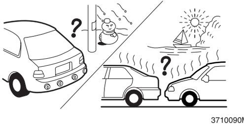
The sensors may not work if the obstacle is an odd shape or made of material that does not reflect ultrasonic waves.
