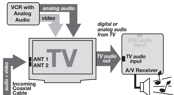
**Setup 1:** A/V receiver audio from the TV's digital or analog audio output (**DIGITAL AUDIO OUT** or **AVR AUDIO OUTPUT**)
