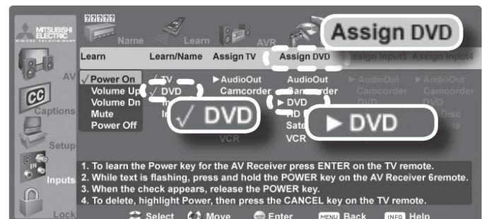
Completed NetCommand setup described for controlling A/V receiver switching to an A/V receiver input labelled “DVD.”
