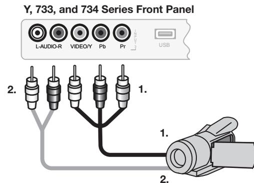
Figure 14. Component video connections for a camcorder
