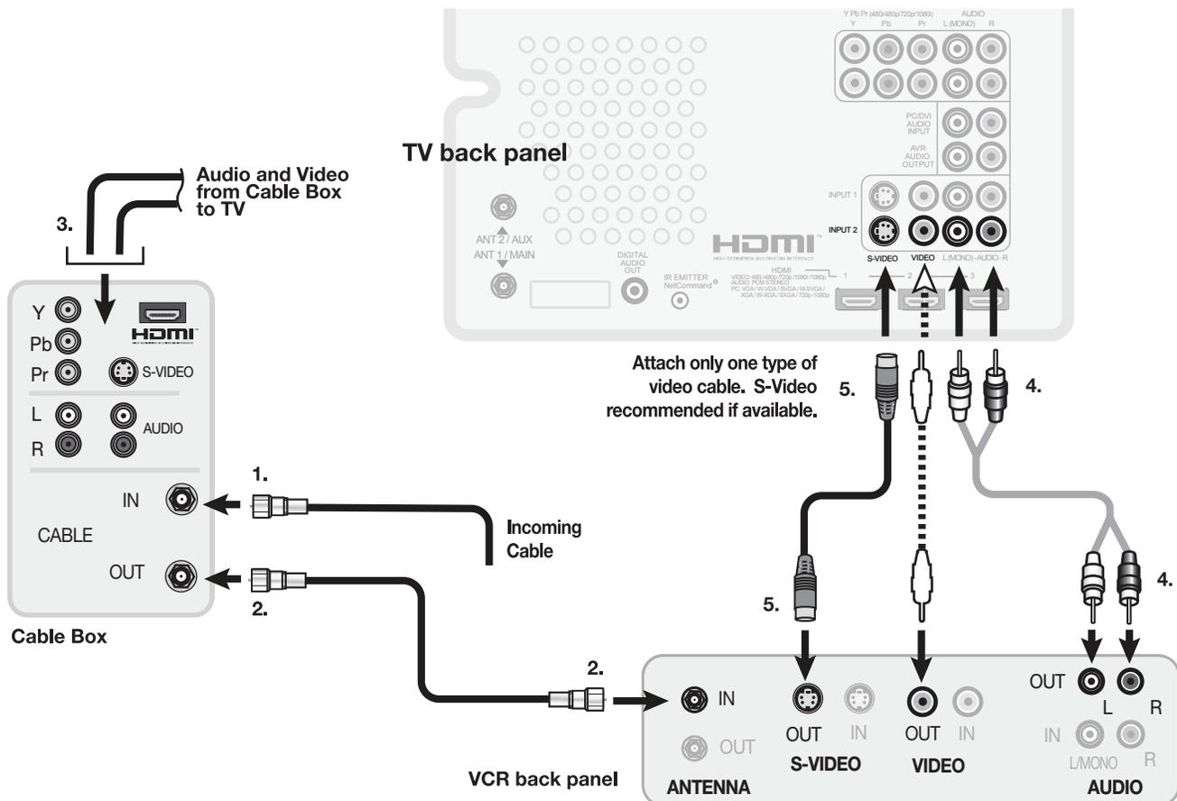
Figure 10. Connecting a VCR to a cable box
