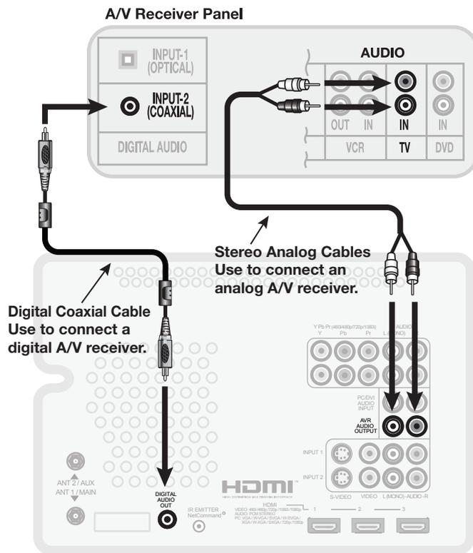
Figure 11. Connecting the TV to an A/V receiver
