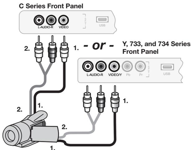
Figure 13. Composite video connections for a camcorder
