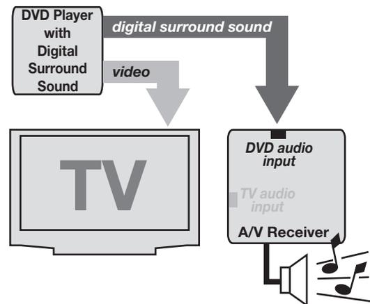
**Setup 2:** A/V receiver audio from a device providing surround sound directly to the A/V receiver
