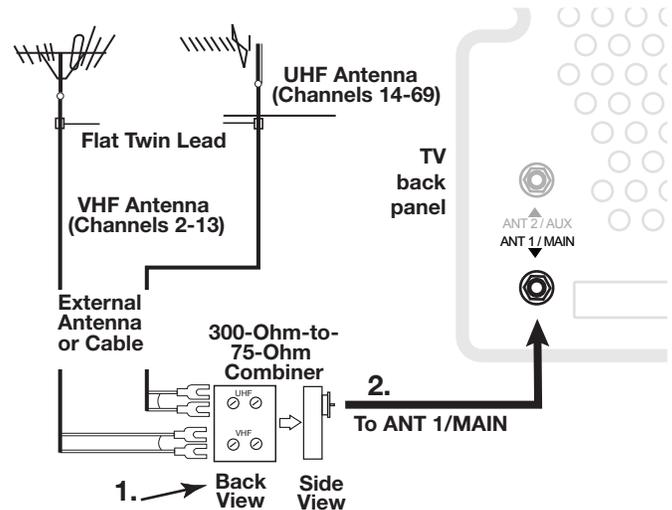
Figure 5. Connecting separate UHF and VHF Antennas
