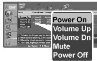
A/V Receiver (AVR) screen. Perform NetCommand IR "learning" for A/V receiver power and volume keys.
