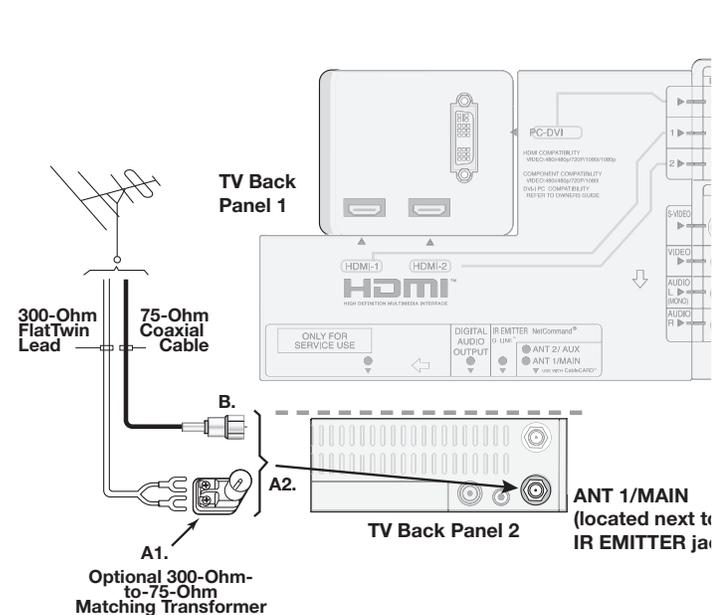
Figure 4. Connecting a Single Antenna
