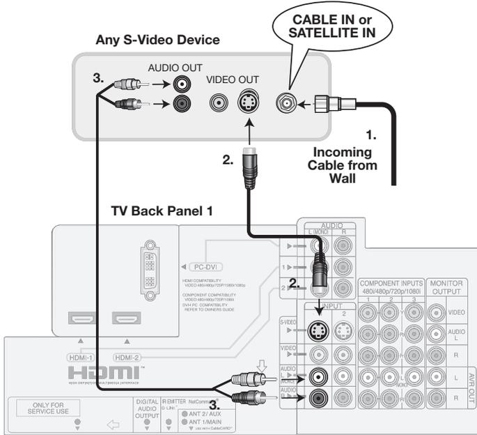
Figure 2. Connecting a device with S-Video
