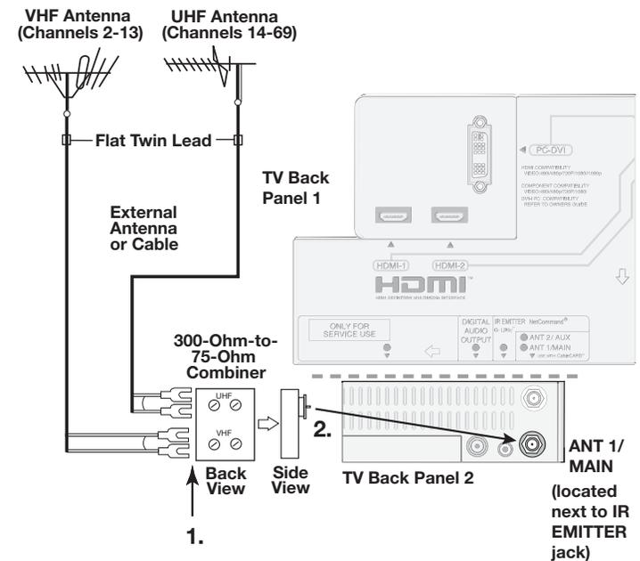
Figure 5. Connecting separate UHF and VHF Antennas
