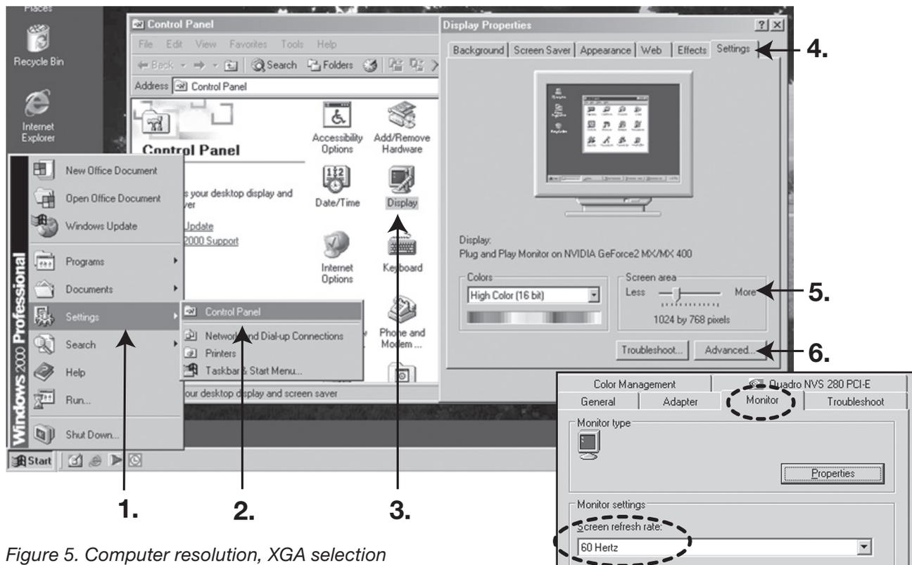
Figure 5. Computer resolution, XGA selection
