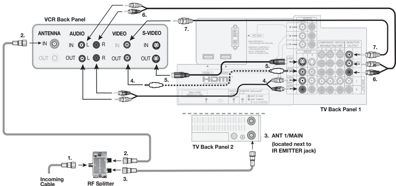
Figure 6. Connecting a VCR to an Antenna or Wall Outlet Cable
