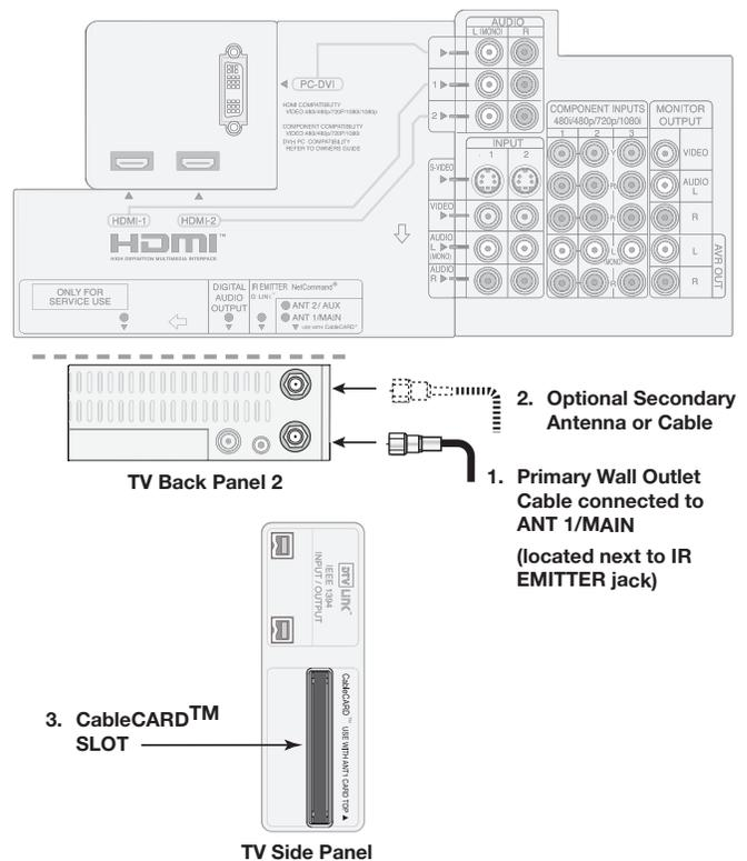
Figure 3. Wall Outlet Cable
