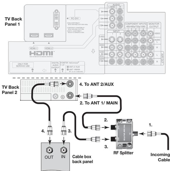
Figure 12. Connecting an older cable box
