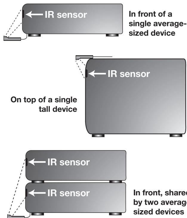
Figure 15. IR emitters so the signal can be "seen" by the IR sensor on each device.
