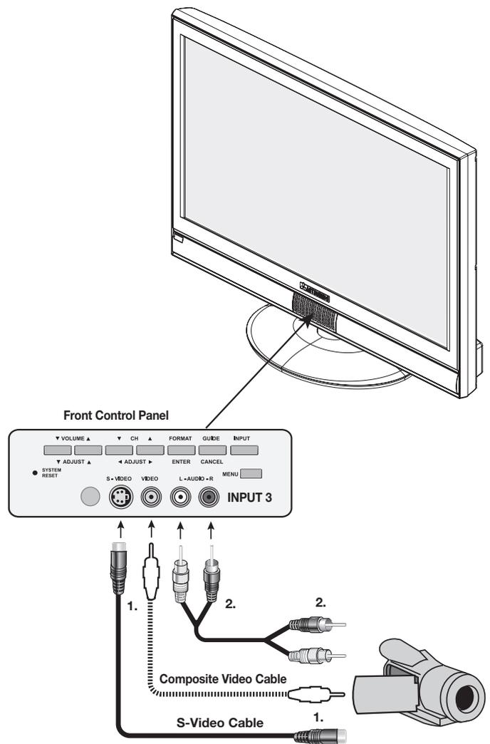
Figure 13. Analog connections for a camcorder
