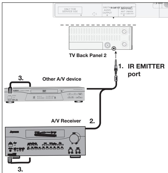
Figure 14. Connecting IR Emitter NetCommand
