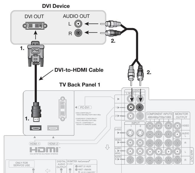
Figure 9. Connecting a DVI device
