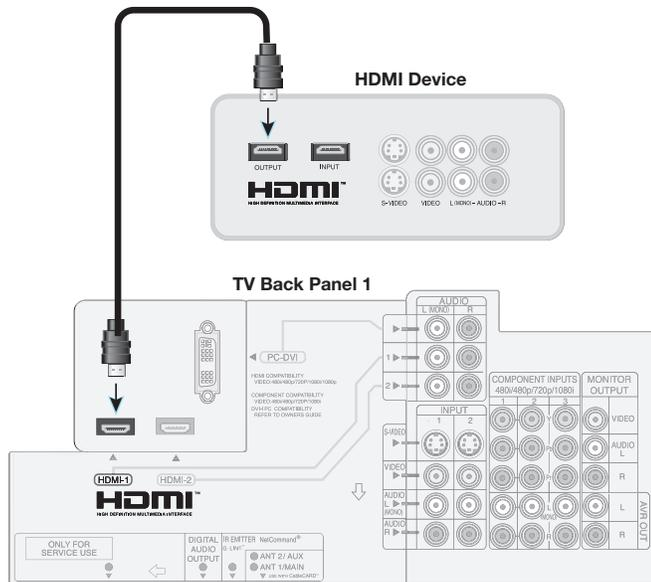
Figure 8. Connecting an HDMI device.
