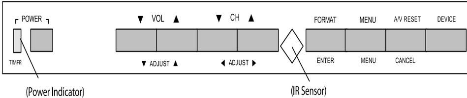
*The ADJUST, ENTER, MENU, and CANCEL buttons may be used to access or navigate through the screen menus*
