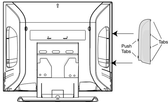
Figure 3. Replacing Input Cover
