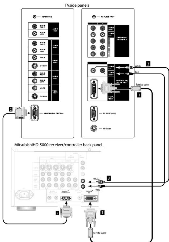
Figure 14. Connecting MonitorLink
