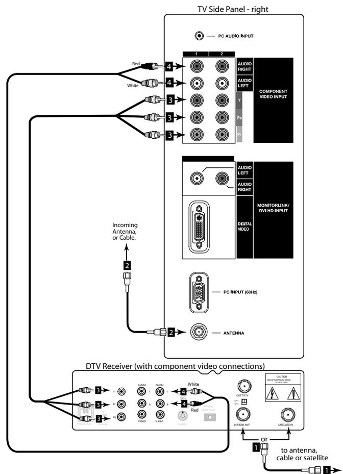
Figure 11. Connecting the DTV receiver with component Video Connections.
