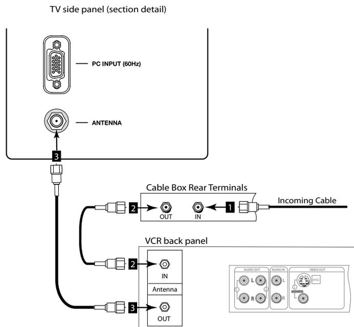
Figure 5. Connecting the VCR with cable box.
