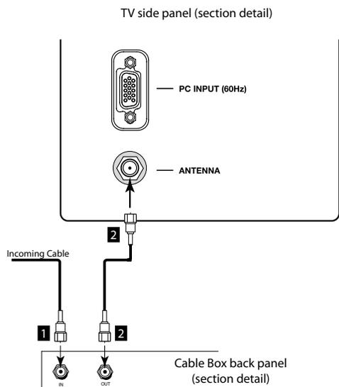
Figure 3. Connecting the cable box.
