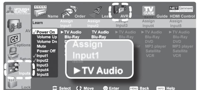
Completed NetCommand setup described for controlling A/V receiver switching to the A/V receiver’s audio input from the TV’s **AUDIO OUTPUT**.
