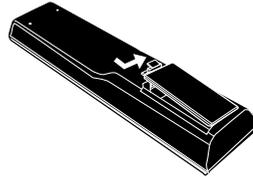
**Step2** Insert two AAA size batteries. Make sure to match the (+) and (-) ends of the batteries with the (+) and (-) ends indicated in the battery compartment. Slide the cover back into place.
