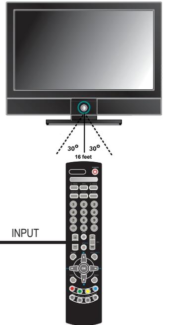
Pressing **INPUT** to display a source list, user **▲/▼** to select the video equipment connected to the video inputs of your LCD TV :TV(CABLE/AIR), VIDEO 1(SIDE), VIDEO 2(REAR), VIDEO 3(S-VIDEO), VIDEO 4(YPbPr1), VIDEO 5(YPbPr2), VIDEO 6(HDMI1), VIDEO 7(HDMI2), COMPUTER(VGA) and press **OK** button.
