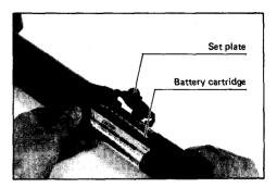
Do not use force when inserting the battery cartridge.
