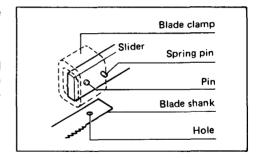
Tighten the bolt securely while making sure that the blade will not be extracted even though you try to pull it out.
