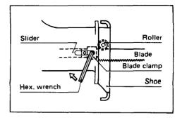
To remove the blade, follow the installation procedures in reverse.
