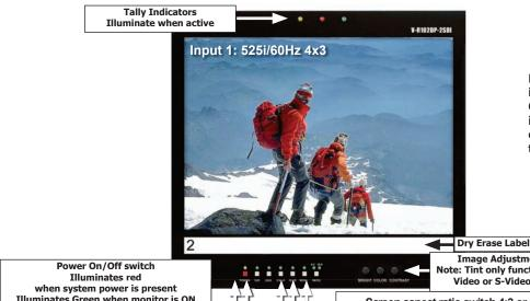
Note: Tapping any active input signal toggles BLUE GUN On/Off. Signal selection is active when Blue Gun is on. Tap active selection to turn off.
