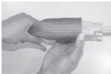
Use the fabric hose included to lay the mains cables, antenna cables or cables from other electronic components systematically; then lead the hose with the cables to the connection boxes. This provides you with an elegant solution when laying cables.
