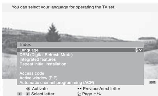
Info on the index item selected is visible at the top of the picture. If the OK symbol is displayed in the line selected, you can use the **OK** button to access the menu directly and carry out settings or selections.
