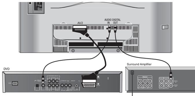
Connect the output socket of the DVD player (DIG OUT) to the TV's "AUDIO DIGITAL IN" socket with a cinch cable.
