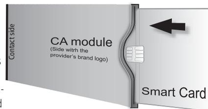
that the side with the golden contact chip faces the side of the module printed with the supplier's brand logo. Printed arrows indicate how to insert the card. Also follow the installation instructions included with the smart card.
