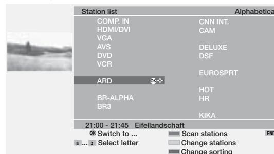
For an alphabetical display: Enter letters with the numeric button (like on a mobile phone keypad), select with  $\blacktriangle \blacktriangleleft \blacktriangleright$  and call with **OK**.
