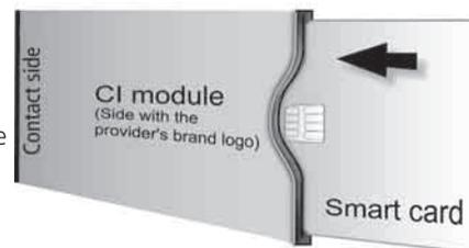
3. Slide the CI module \* carefully into the slot with the contact side facing the front. The logo on the common interface module should be visible. Make sure the module is not twisted in the process. Do not use force. When the module locks, the eject button is pressed outwards.
