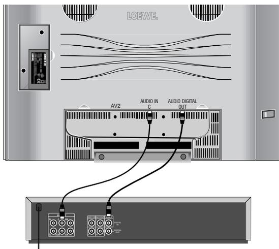
Select “Analogue” for “Sound transmission” for **analogue audio amplifiers**. The sound for the analogue amplifier is transmitted via the AUDIO OUT L/R connections of the TV to the audio amplifier. Connect the amplifier with two cinch cables.
