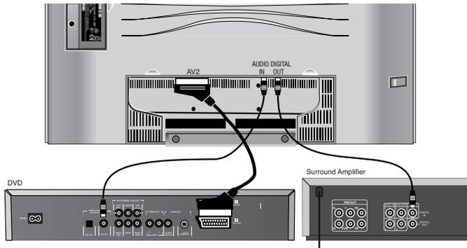
Connect the output socket of the DVD player (DIG OUT) to the TV's "AUDIO DIGITAL IN" socket with a cinch cable.
