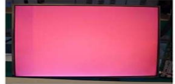
Vertical Block Source TAB IC Defect
