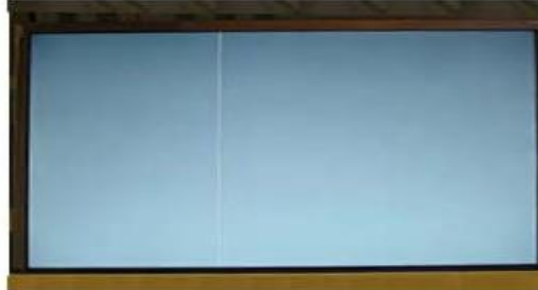
Vertical Line Source TAB IC Defect
