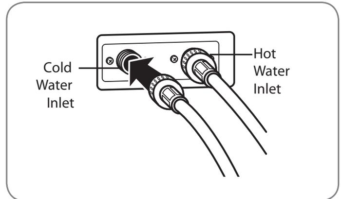
4. Attach the (red) hot water line to the hot water inlet on the back of the washer. Attach the (blue) cold water line to the cold water inlet on the back of the washer. Tighten the fittings securely.
