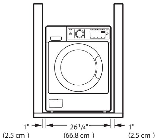
Allow at least 21 1/4 in. (54 cm) in front of the washer to open the door.
