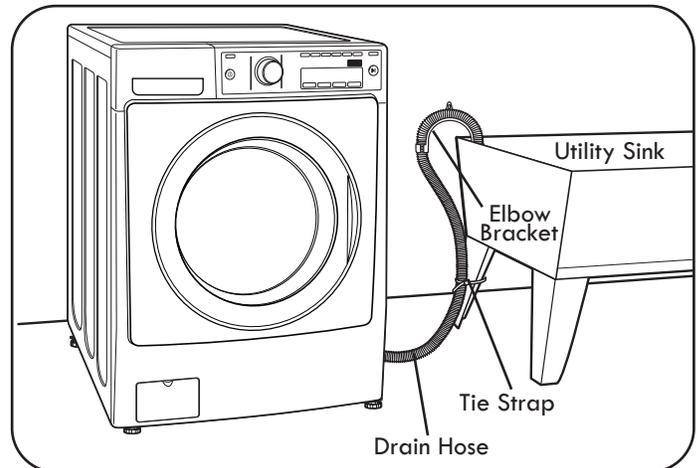
The elbow bracket should be installed near the end of the drain hose. Hang the end of the drain hose over the side of the utility sink. Use a tie strap to secure the drain hose in place.
