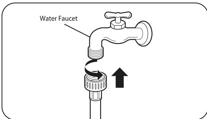
2. Connect the water supply hoses to the HOT and COLD water faucets tightly by hand and then tighten another  $\frac{2}{3}$  turn with pliers.
