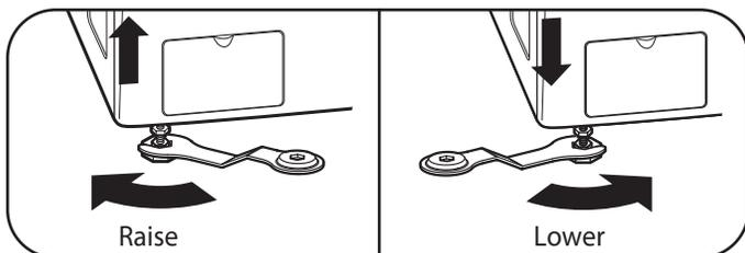
2. Loosen the locknuts on all four leveling feet with the wrench until you can adjust the feet (wrench appearance may vary). Use the wrench to turn the feet clockwise to raise the washer, and counterclockwise to lower the washer. Using a level, adjust the feet until the washer is level from side to side and front to back. Make sure that all four feet are in firm contact with the floor.
