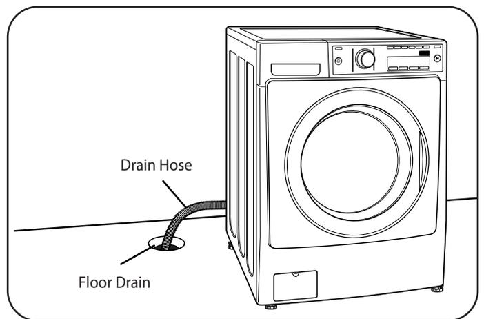
Insert the end of the drain hose into the floor drain. If possible, secure the hose to prevent it from moving or coming out of the drain.
