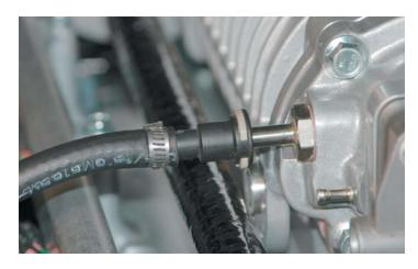
88. Locate the Vacuum accessory line at the fire wall and install the length of 1/8 hose supplied onto the end of the check valve.
