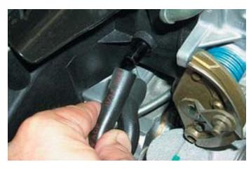
20. Disconnect the eight fuel injector connectors by pulling up on the grey release latches and the squeezing them at the top. Remove the injector harness clips from the intake manifold.
