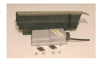
158. Assemble the Magnavolt unit to the Fuse/Relay center cover by placing the rubber mounts into the two holes in the cover and then place the magnavolt on the rubber mounts. Secure the mounts with the nuts supplied and tighten them with a 10mm wrench.
