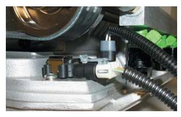
80. Install the eight Injector Wiring Adaptors on to the harness fuel injectors connectors.
