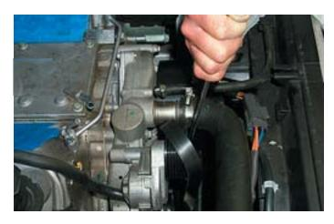
40. Remove the stock belt tensioner assembly by removing the two mounting bolts with a 15mm socket wrench.
