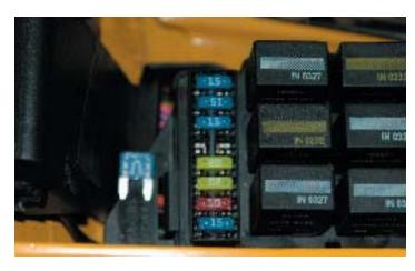
128. Place one leg of the 15 amp fuse through the Fuse-Tap supplied.
