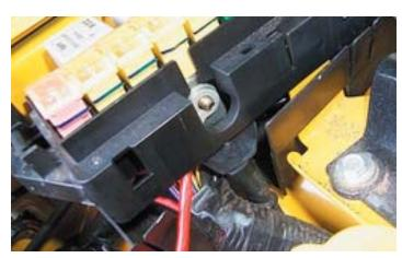
132. Lay the coolant pump relay next to the row of fuse on the Fuse/Relay center base. Install the Fuse/Relay center cover on the base by raising the relay slightly to hook the rear edge of the cover on the base then snap the cover in place.
