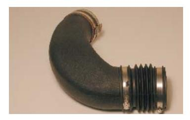
104. Attach the bellows end of the air tube on the air meter.
