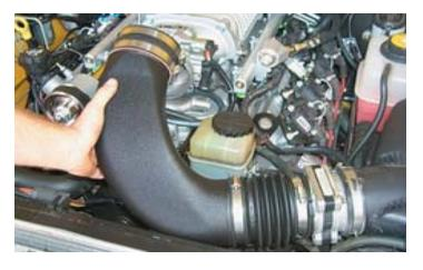
105. Attach the hose end of the air tube to the throttle body. Tighten all clamps securely.
