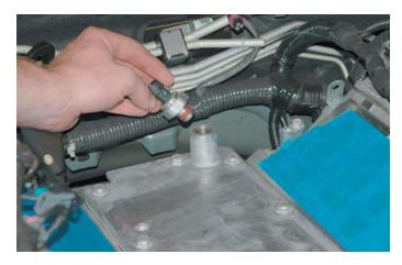
44. Remove the engine valley cover and gasket by removing the ten bolts with a ratchet and 13mm socket.
