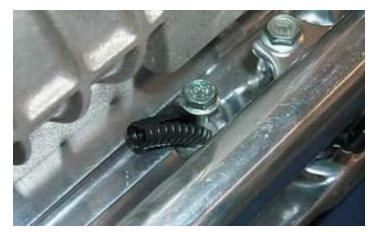
75. Torque all ten bolts that secure the manifold to the cylinder heads gradually and evenly to a torque of 89 in-lbs. Use a 10mm socket and torque wrench.
