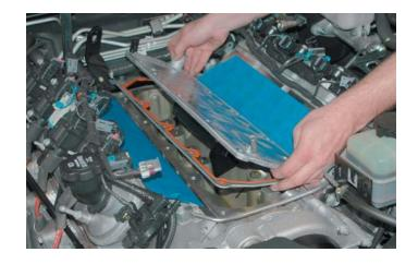
46. Using a small straight blade screwdriver, remove the 8 O-rings from the underside of the engine valley cover and transfer them to the grooves in the bottom of the new cover.
