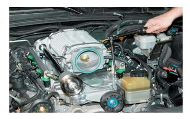
76. Install the throttle body onto the new inlet manifold with the original mounting bolts. Torque the mounting bolts to 106 in-lbs.
