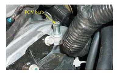
110. Insert the new check valve into the 11/32" brake hose.
