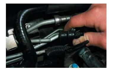
26. Remove the EVAP tube connector from the intake manifold by pushing in on the white release trigger and pulling firmly.
