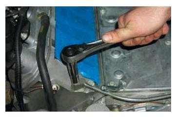
36. Remove the coolant vent pipe. Ensure that the Oring gaskets under the vent pipe blocks do not stick to the cylinder heads. If so, remove them as new gaskets are supplied.
