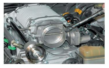
77. Ensure that there is clearance between the transmission fill tube and the fuel cross-over pipe.
