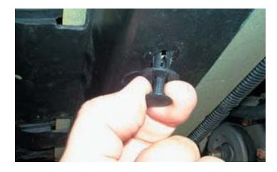
114. Remove the five push-lock fasteners and the radiator shield.
