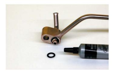
38. Install the new vent pipe with the supplied bolts and torque them with a torque wrench and 10mm socket to 106 in-lbs.
