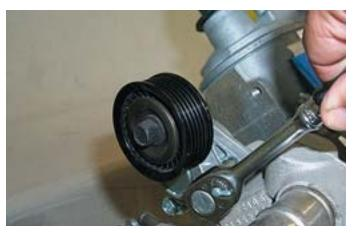
41. Install the new tensioner assembly in place of the stock unit with the supplied bolts and torque them to 40 ft-lbs.
