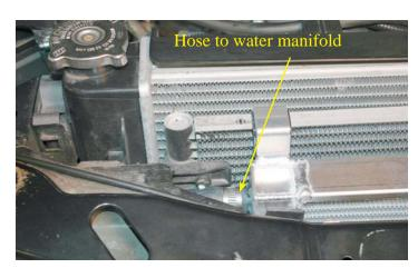
152. Using the remaining hose cut from the molded 90 degree "elbow" hose, trim this piece to 13" long and install it onto the right barb on the intercooler water manifold. Connect the other end to the upper barb on the intercooler reservoir. Secure the hose with #10 clamps.
