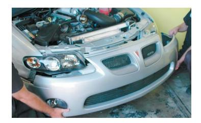
154. Replace the upper radiator and lower splash shields with the push-lock fasteners that secure them.
