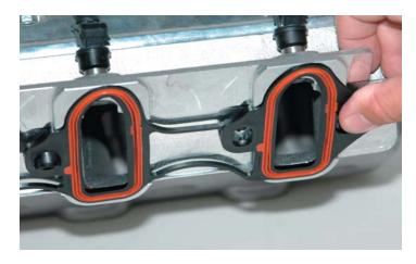
72. Remove the tape from the ports. Use silicone or some mild soap and water solution to lubricate the port surfaces. This will help align the manifold and bolt holes. (Do not use anything that will damage the silicone port gaskets.)
