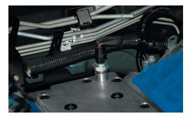
51. Remove the engine lift bracket from the rear of the right cylinder head by removing its two mounting bolts with a 15mm wrench.
