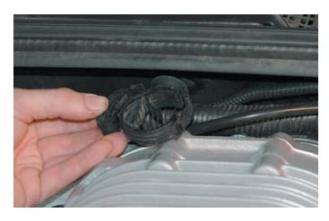
176. Here is the new harness clamp assembly, it will mount in the rain gutter hole that you removed the screw from in the previous step.
