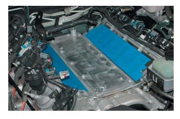
45. The gasket will be reused, the original valley cover and bolts will not. Inspect the gasket for any damage and then reinstall, note that it will only fit correctly in one position.
