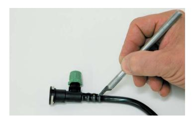
84. Using the piece of 5/16" EVAP hose supplied cut it into two pieces. One piece 28" long and the other 16" long. (The hoses are shown shorter for clarity.) Starting with the longer of the two, assemble the hose with the test port on one end and the right angle on the other using the #6 clamps supplied. On the remaining hose, assemble it with the straight fitting, squeeze fitting and clamps.
