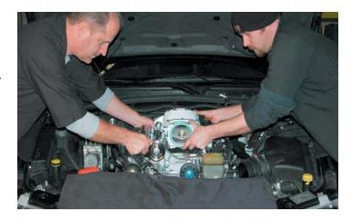
74. Remove the split-looms that support some of the manifold to cylinder head bolts. Start all ten bolts by hand to ensure proper alignment of the manifold.
