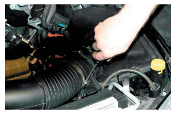
15. Loosen the Air Tube clamp at the throttle body.
