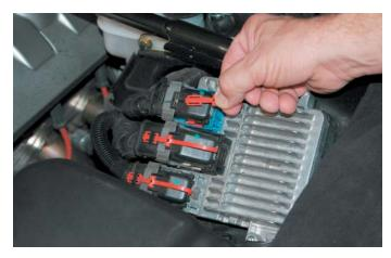
4. There are three computer connectors, Grey, Black and Blue. Remove the connectors by first removing the Red locking key, then pushing in on the Black cover and pushing the Grey latch down to open it.
