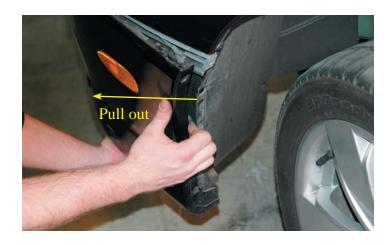
118. Push the front fascia forward and then pull out at the edge of the fascia below the head light on both sides to free the locking tab.
