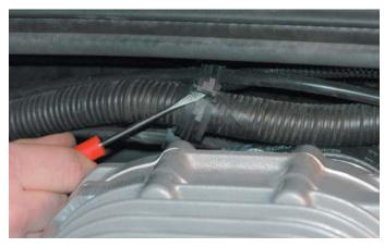
175. Remove the harness clamp from the firewall, it will not be re-used.
