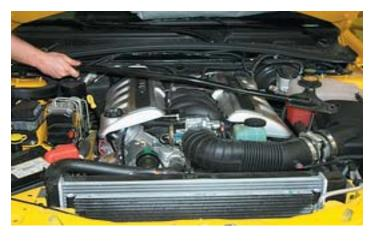
13. Remove the two engine covers by pulling up firmly along the edges.
