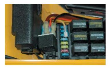
133. Route the pump harness and connector down to the pump through the harness hole next to the battery platform.
