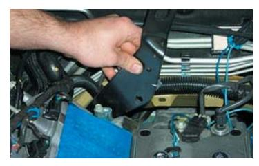
52. The automatic transmission fill tube will need to be moved slighly outward to avoid contact with the supercharger fuel cross-over pipe.
