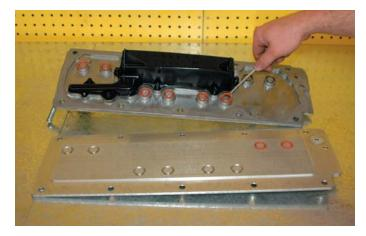
47. Install the new engine valley cover and flathead bolts supplied with a 5mm Allen socket and torque the bolts to 18 lb-ft. Insert the six O-rings in the recesses in the new valley cover.
