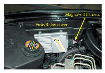
162. On the passenger side shock tower, locate the circular wire conduit. Cut the Ty-strap where it meets the Fuse/Relay center. Using a small straight blade screwdriver, genly pry the locking tabs free on the upper cover of the conduit to free the cover.
