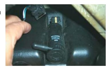
123. Remove the bolt that secures the rear of the reservoir bolt with a 10mm socket wrench.
