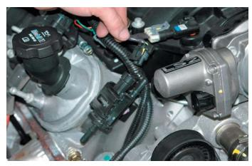
25. Remove the EVAP line at the firewall by squeezing on the connector and pulling it free.
