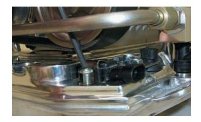
70. Install the fuel manifold O-ring into the recess on the fuel rail with some of the grease supplied. Next install the fuel manifold using a 4mm Allen socket and torque wrench. Torque the manifold fasteners to 106in-lbs.
