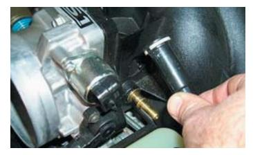
27. Remove the vacuum acessory hose and connector from the rear of the manifold.
