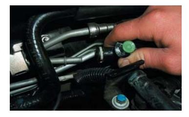
86. Re-connect the Purge solenoid electrical connection, then install the right angle fitting of the long EVAP hose to the top connection of the Purge solenoid. Connect the squeeze fitting of the shorter EVAP hose to the lower connection of the solenoid.
