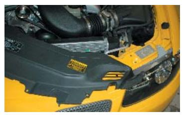
115 Remove the three screws that secure the front fascia or "nose" of the vehicle with a cross-head screwdriver.
