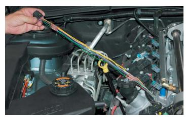
95. Cover the extended ETC harness with the new split loom supplied. route the extended harness under the throttle body and install the connector onto the throttle body
