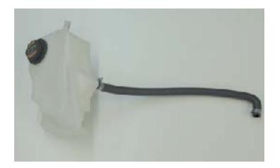
146. Place the intercooler reservoir on the top of the battery. Ensure that the Velcro has a good "grip".
