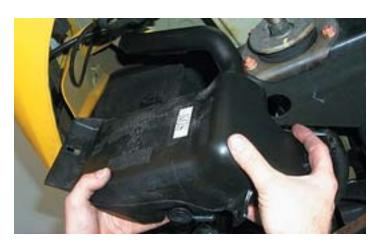
136. Make a hole in the passenger side of the splash shield as shown for the intercooler coolant hoses to reach the heat exchanger.
