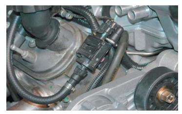
87. Connect the remaining end of the short EVAP hose to the fitting on the passenger (left) side of the inlet manifold above the supercharger drive shaft.
