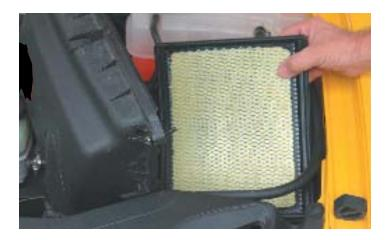
100. Replace the stock filter element with the K&N air filter element supplied.
