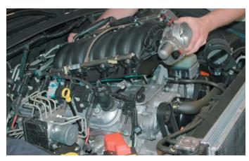
32. Use a shop vacuum cleaner to remove any debris or dirt from the intake port area and engine valley cover.
