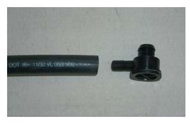
111. Install the check valve into the grommet on the brake booster.
