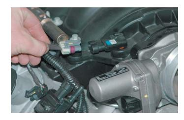
22. On both sides of the engine disconnect the ignition coil pack connectors from the coil packs by first removing the blue lock key.
