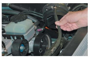
92. Route the vent line down under the tensioner mounting bracket to the steam vent pipe barb. Trim the vent hose to length and attach it to the vent pipe barb.
