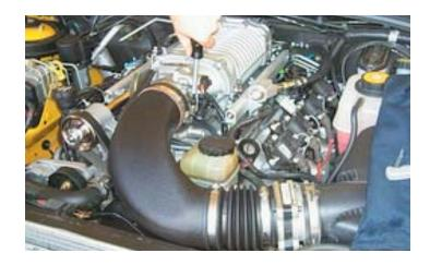
106. Install the PCV inlet hose. Cut a 16" length length of 3/8" hose supplied and attach one end to the barb on the right valve cover. Attach the other end of the hose to the barb on the bottom of the new air tube.
