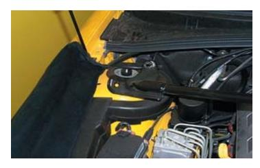
12. Remove the strut tower brace and fasteners from the vehicle, the brace can be reinstalled after the supercharger installation.
