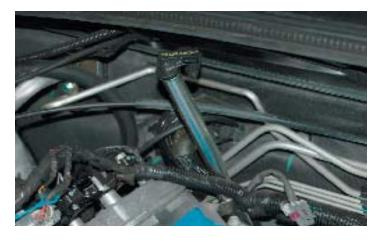
53. Vehicles with automatic transmission only. Manual transmission vehicles please skip to step the next. Move the automatic transmission fill tube by pulling it firmly outward towards the fender of the vehicle. It will only be necessary to move the tube 1/4"-3/8". After installing the supercharger and manifold assembly, check for contact between the fill tube and the fuel cross-over pipe.
