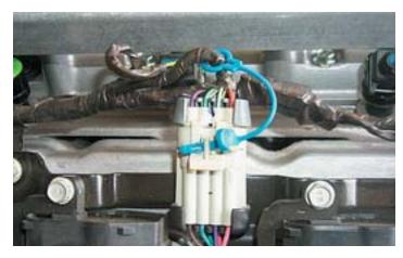
79. At the rear of the supercharger on the passenger side, plug in the new MAP and IAT connections.
