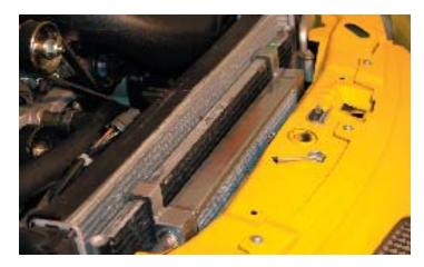
148. Install the two 6x20mm bolts through the power steering cooler bracket and into the lower brackets on the heat exchanger. You can access these bolts through the lower grill or by pulling down the lower splash apron. Tighten the two bolts securely with a 10mm socket wrench. Replace the radiator shield and 5 push-lock fasteners.
