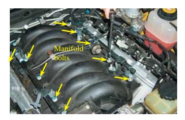
31. Remove the intake manifold, fuel system and throttle body assembly.
