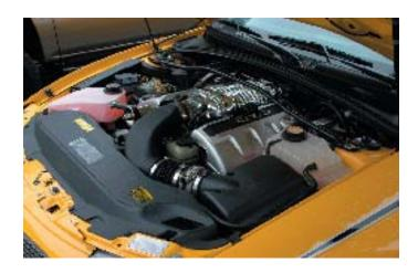
180. Starting with the right side engine cover, trim the cover as shown using a small saw. Go Slow! The plastic of the covers will cut very easily and a professional result can be achieved with a little patience. Test fit the covers as you go. Finish the cut edges with a file and sandpaper.
