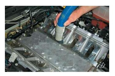
33. Cover the intake ports with tape or clean rags to keep dirt and debris from entering the engine.
