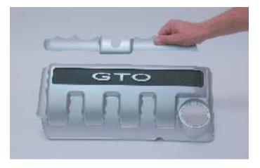
181. On the left side engine cover trim the cover as shown. A little more care must be used on trimming this cover as you must make room for the bypass canister. Trim and test the cover fit several times to get a good fit and finish. Leave the finished covers off the engine until you have completed your test drives and final inspection.
