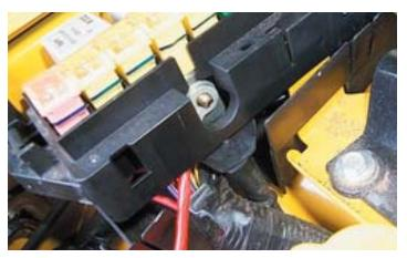
161. Replace the cover with the Magnavolt attached on to the Fuse/Relay center. Connect the Magnavolt harness to the unit.
