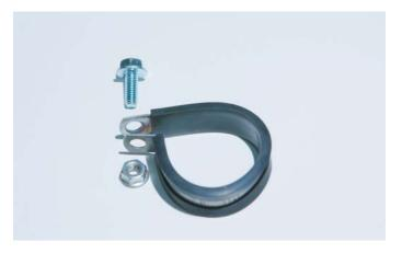
177. Install the harness clamp around the harness, hoses and cables directly behind the supercharger assembly. Take care that nothing can come in contact with the rear drive belt and pulleys. Secure the new clamp with the supplied bolt and nut in the rain gutter hole. Tighten them securely with a 10mm wrench.
