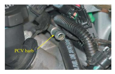
108. Install the plain end of the 18"PCV outlet hose on the passenger (right) side of the engine.
