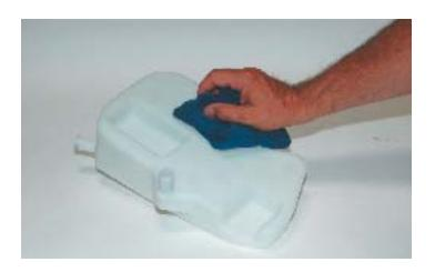
142. Cut the 15" length of Velcro supplied into six pieces 2-1/2" long. Peel off the paper backing and install three pieces of Velcro onto the bottom of the reservoir as shown.
