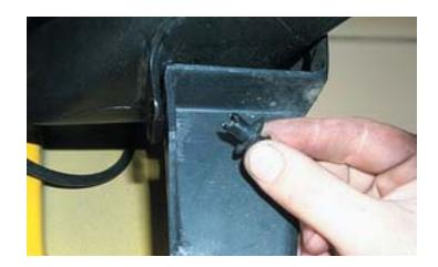
126. Remove the reservoir by rotating it 90 degrees and lowering it down and out.
