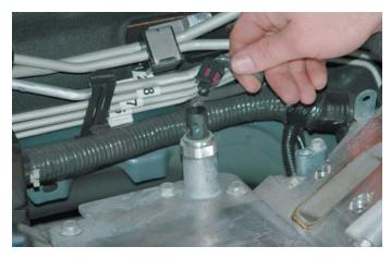
43. Remove the engine oil pressure sensor from the valley cover with a 28mm wrench.
