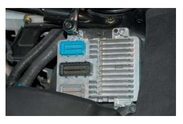
172. Carefully replace the three computer connectors by pressing them in place and pushing grey larches back into place untill they snap into their original locations on the black covers. Secure the connectors with the red locking keys.
