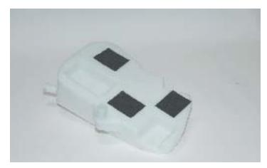
143. Re-install the battery and its connections. Using the reservoir as a guide attach three pieces of Velcro to the top of the battery.
