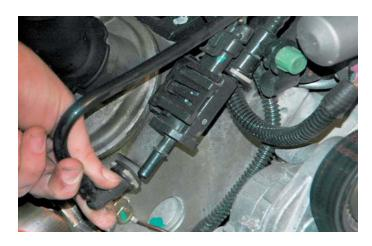
24. Disconnect the Evaporative Purge Solenoid (EVAP) electrical connector.
