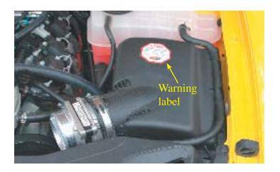
102. Here is the new air tube and mounting components.
