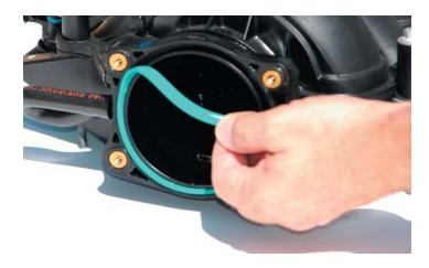
56. Install the throttle body O-ring into the groove on the new inlet manifold. The LS2 throttlebody will be installed after the supercharger assembly is installed on the engine.
