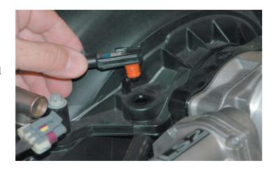
68. Apply a small amout of the grease supplied to the MAP sensor seal and install the sensor in its new location at the right rear of the supercharger manifold.
