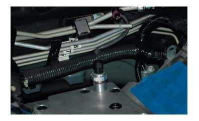
50. Re-install the oil pressure sensor and torque it to 15 ft-lbs. Re-attach the sensor electrical connector.
