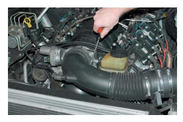
16. Remove the PCV tube from the air tube and from where it connects to the valve cover barb.
