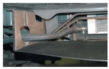
151. Route the hose from the upper barb down through the new hole in the right side of the splash shield. Continue the hose up into the engine compartment and connect it to the rear barb of the water manifold. Secure the hose with #10 clamps.
