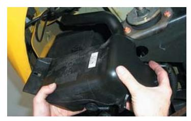
127. Install the intercooler pump relay harness by removing the cover of the Fuse/Relay center on the right hand side of the engine compartment. Remove the fourth 15amp fuse from the top marked "AUTO TRANS" temporarily from the base.
