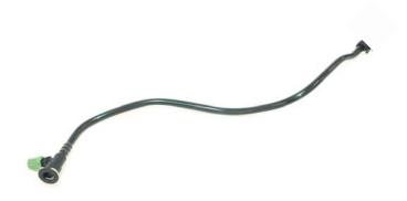
83. Using a sharp shop knife, cut the hard plastic tube where it covers the the barbed end of the EVAP fittings. Take care not to damage the fittings as they will be reused.
