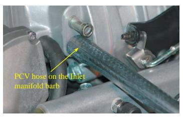
109. At the rear of the left valve cover, remove the black rubber cap from the PCV barb. Connect the end of the PCV outlet hose to this barb.
