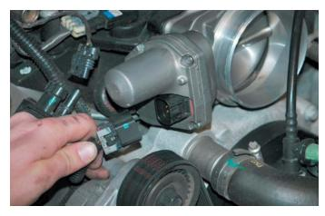
19. Remove the PCV hose that connects the intake manifold to the engine valley cover vent.
