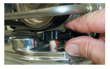
69. Install the MAP sensor in its new location using the supplied bracket and the button head Allen screw with a 4mm Allen wrench.
