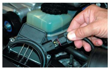
59. Remove the tape and split loom from the harness to about 6" below the MAF connector. Locate the Brown/Yellow and the solid Brown wires. These are the Intake Air Temperature (IAT) sensor wires on the connector. Cut these two wires approximately 2" below the connector.
