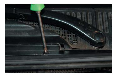
174. Using a small straight blade screwdriver, open the harness clamp and pull the harness free.
