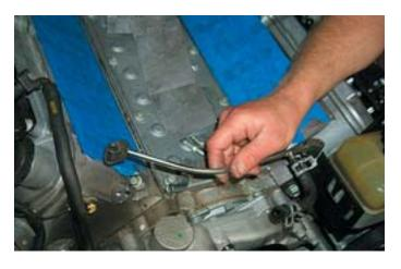
37. Install the new vent pipe O-ring gaskets using the supplied grease to hold them in place.
