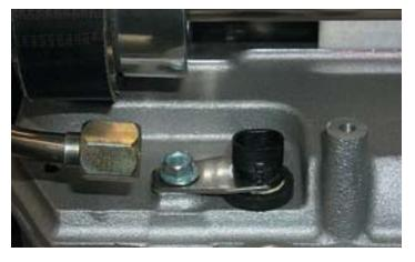
65. Locate the MAP connector on the harness. Remove the black tape and split loom from the MAP connector and wires. Viewing the connector from the top or clip side note the location and colors of the three wires on the connector, Purple/White left, Green center and Black on the right. Approximately 1" behind the connector cut these three wires.
