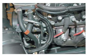
63. Install the IAT sensor (supplied for LS2) into its location at the right rear corner of the supercharger manifold. (Fuel rail and injector removed for clarity.) Apply a small amount of the supplied grease to the body of the sensor. Lift the manifold bolt and retaining bracket to slide the IAT sensor into the mounting grommet.
