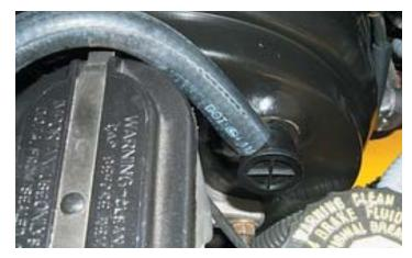
112. Connect the end of the brake booster hose to the upper barb on the driver side of the inlet manifold.
