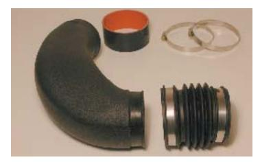
103. Install the hose connector and bellows on the air tube with the clamps supplied.
