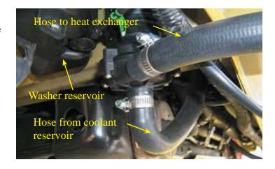
150. Connect the hose from the lower heat exchanger barb to the outlet on the pump through the new hole in the splash shield. Secure the hose with #10 clamps.
