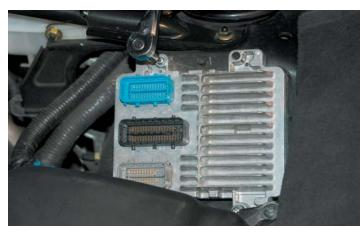
7. Remove the computer carefully from the vehicle.
