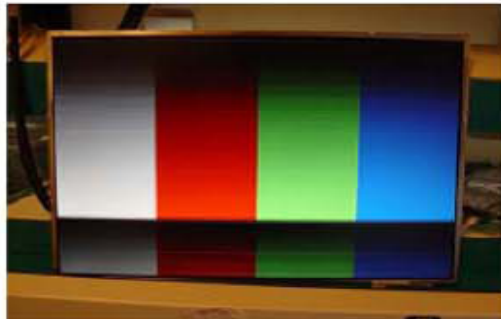
Horizontal Block Gate TAB IC Defect
