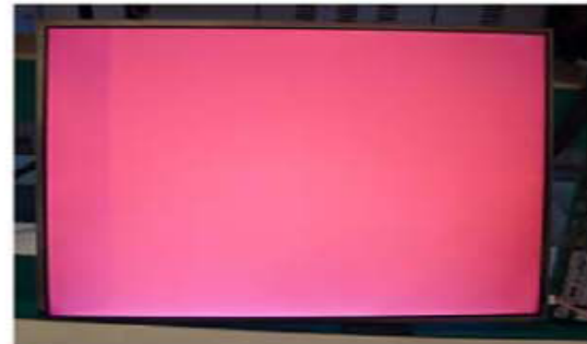
Vertical Block Source TAB IC Defect
