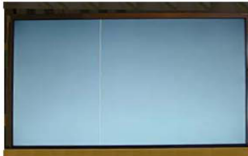
Vertical Line Source TAB IC Defect
