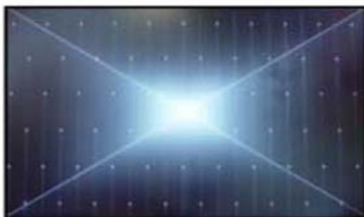
Solder defect, Short/Crack
