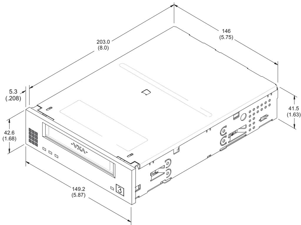
**Figure 7-1** Physical dimensions of the internal tape drive
