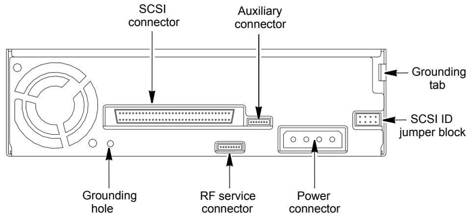
**Figure 2-1** Internal SCSI tape drive: back-panel components
