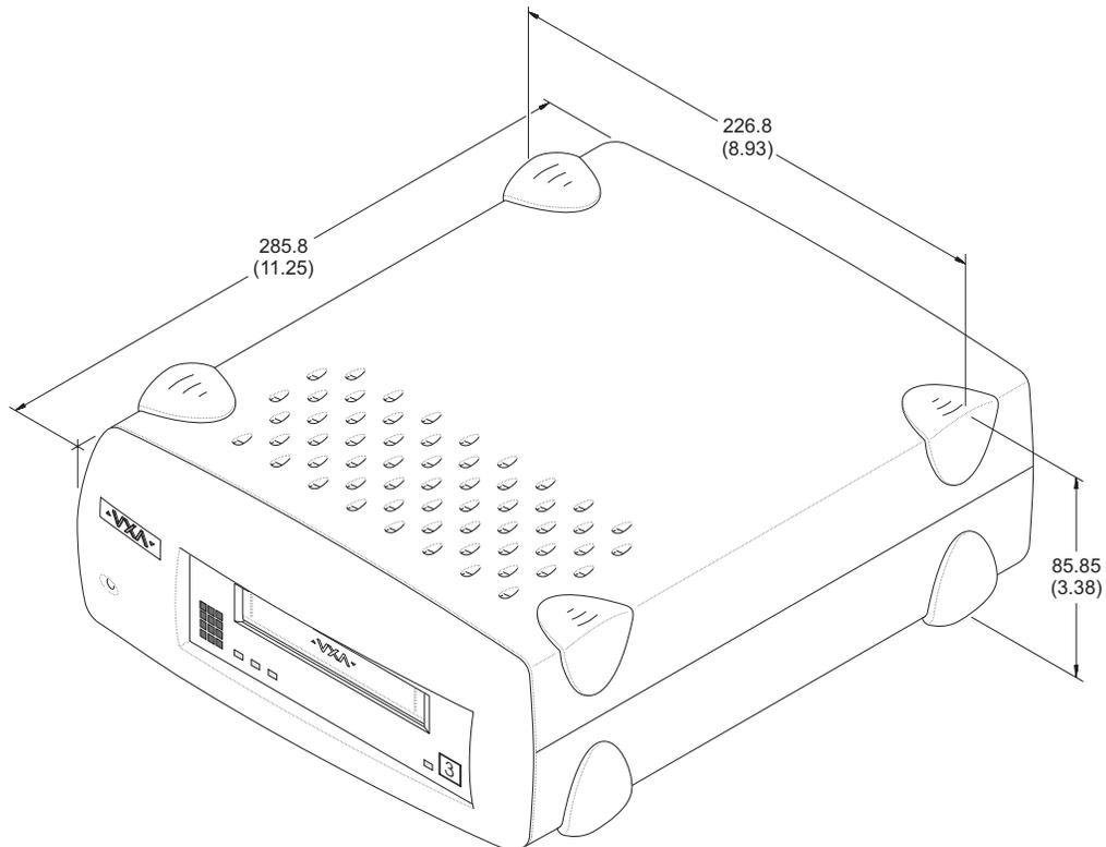
**Figure 7-2** Physical dimensions of the external tape drive
