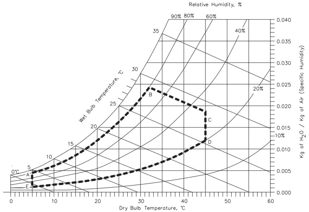
**Figure 7-3** Internal model: Operating temperature and humidity ranges
