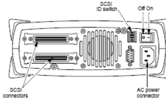
**Figure 1-5** External tape drive: back-panel components
