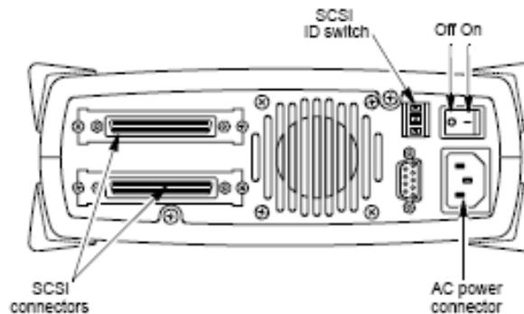
**Figure 2-6** External SCSI tape drive: back-panel components
