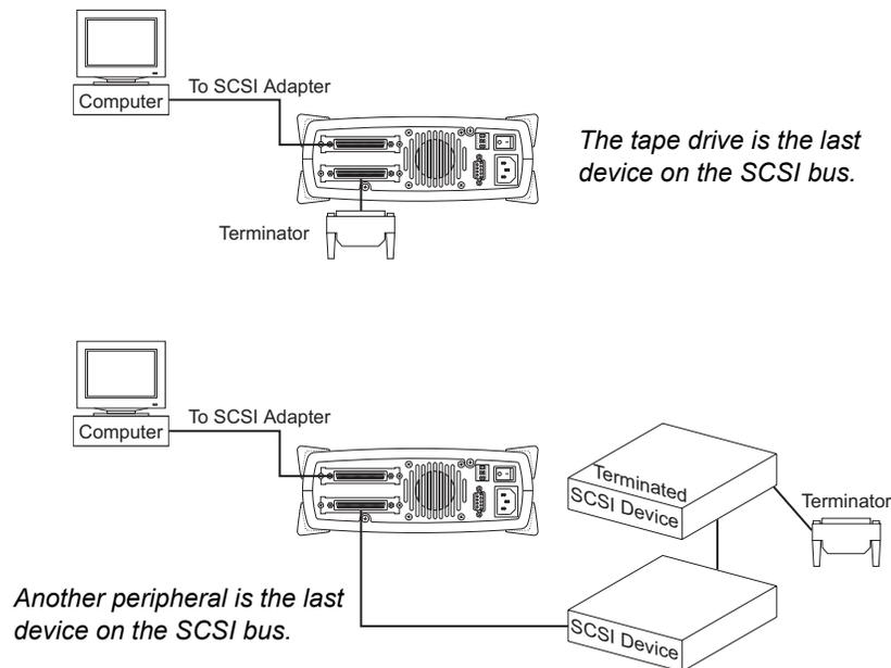
**Figure 2-7** Terminating the SCSI bus (external model)
