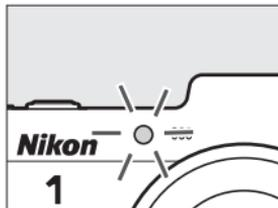
**Remote control mode:** Aim the ML-L3 at either of the infrared receivers on the camera (📖 2, 3) and press the ML-L3 shutter-release button (stand at a distance of 5 m/16 ft or less when using the front receiver, 1.5 m/5 ft, or less when using the rear receiver). In delayed remote mode, the self-timer lamp will light for about two seconds before the shutter is released. In quick-response remote mode, the self-timer lamp will flash after the shutter has been released.
