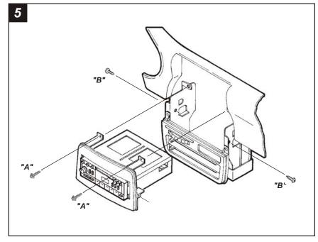
Re-connect the battery terminal and test the unit for proper operation. Mount the head unit/kit assembly to the sub-dash with (2) 7mm hex-head screws previously removed in step #1 ("A") and (2) #10 Phillips screws supplied ("B").
