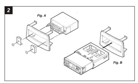
**2-SHAFT HEAD UNITS:** Snap the **Shaft Supports** into the **Radio Housing.** Slide the aftermarket head unit into the kit and secure with shaft nuts. (see Fig. A)
