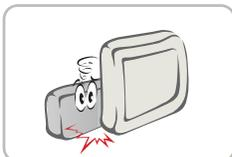
Be careful the battery pack terminals do not short circuit.
