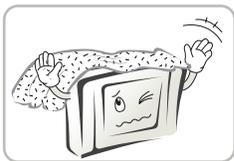
Ensure that ventilation openings are not blocked by a tablecloth, curtain or similar material.
