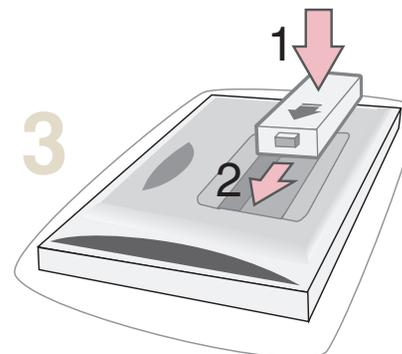
Insert the battery pack down into the battery pack holder (1), then slide it left (2).
