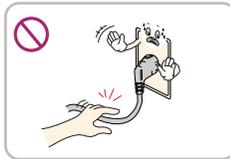
Hold the plug with your hand when pulling out the power cable. Do not bend the cord with excessive force, or put a heavy object on it.
