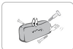
Do not keep the battery pack close to a metallic object like a key or a clip.
