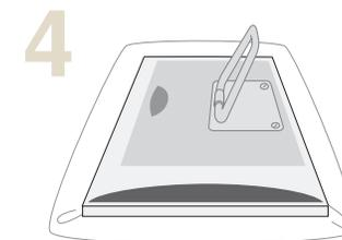
Replace the cover and screws after installing the battery pack.
