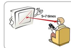
Viewing distance from the product should be about 5 ~ 7 times of the diagonal distance of the screen.
