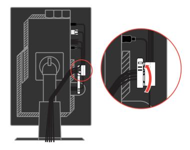
Wrap the Cable Wrapper around the cables.
