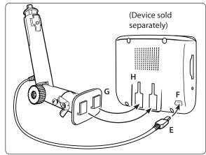
Step 2. Attach the device to the pedestal by inserting the dual T-tabs of the pedestal (G) into the dual T-slots of the device (H).
