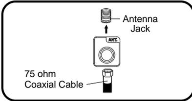
For basic Cable TV service not requiring a Converter/Descrambler box, connect the 75 ohm Coaxial Cable directly to the Antenna Jack on the back of the TV.
