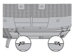
• Leave the cover off if they do not fit properly. Do not force to replace the cover. Doing so may cause damage to the connection cables and the cover.
