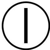
**ON** - Pressing this button for four seconds will start the UPS.
