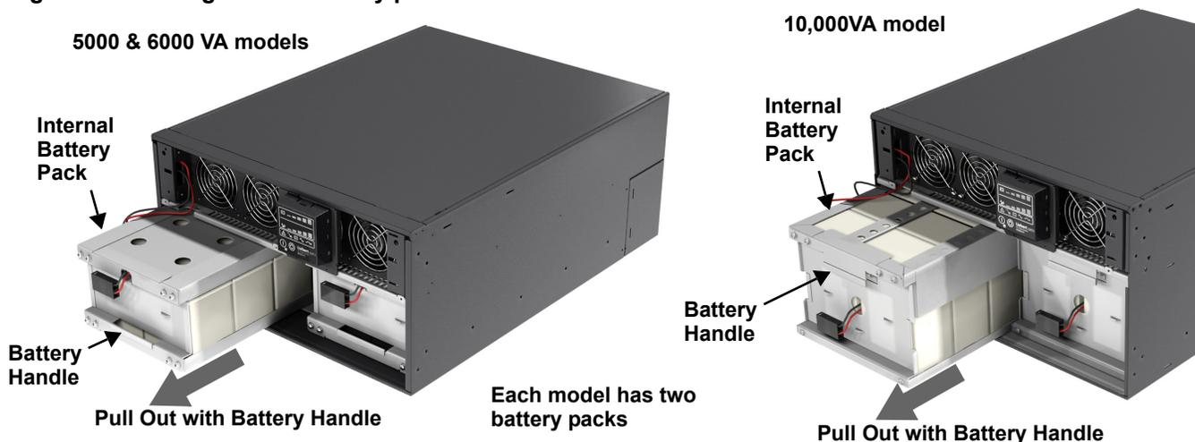
6. Unpack a new internal battery pack. Take care not to destroy the packing. Compare the new and old internal battery packs to make sure they are the same type and model. If they are the same, proceed with **Step 7**; if they are different, stop and contact your local Emerson® representative or Emerson Channel Support.
