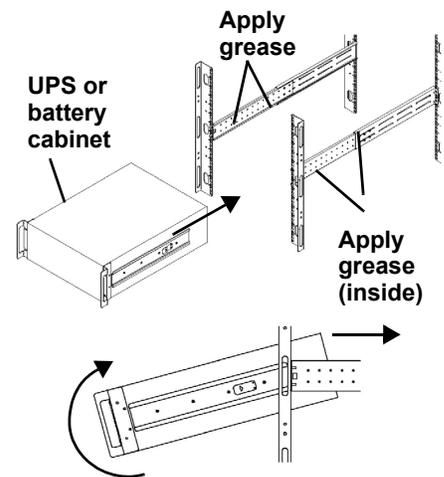
**Insert the UPS into the front members, lift the front and push it into the rack.**
