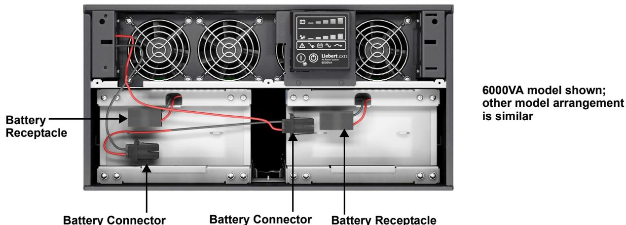
5. Grasp the battery handle and pull one of the internal battery packs out of the UPS, as shown in **Figure 19**. Repeat this step if both battery packs will be replaced. Each model has two battery packs
