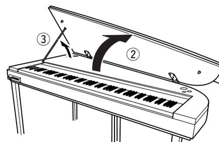
3. Raise the lid stay and carefully lower the lid so that the end of the stay fits into the recess in the lid and holds it in place.
