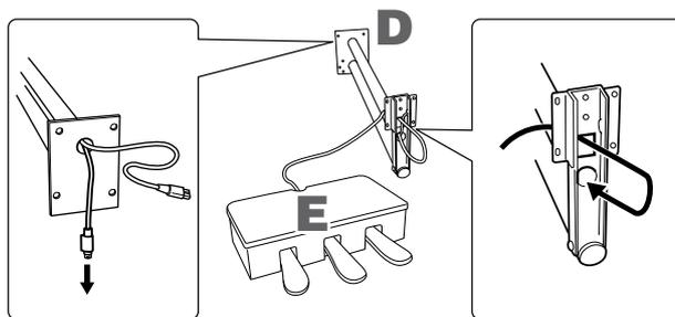
**5-2** Align the holes on the bottom of E with the holes on the bracket of D, then attach E and D by tightening six small screws (4x6 mm). At this time, first tighten the two center screws, then tighten the rest of the screws.
