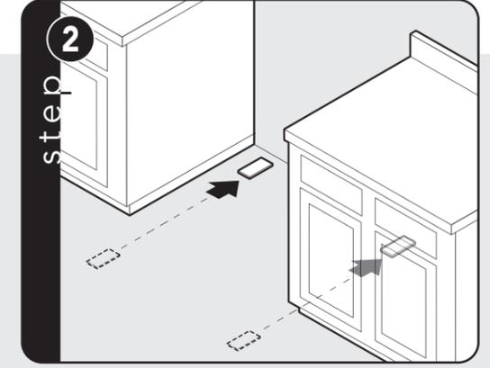
For uneven or sloped floors, level unit with metal shims only, as the adjustment required may exceed the thread available in the leg.
