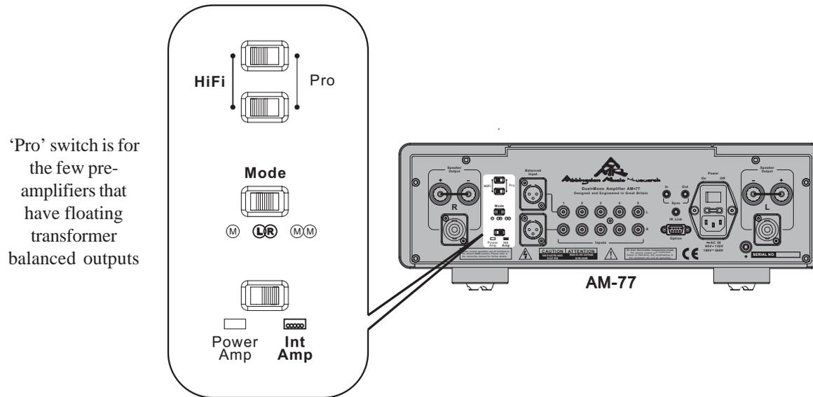
For the majority of sources, the HiFi/Pro switch (R3) is best left in the 'HiFi' position. However, if the source has a pro-audio style transformer balanced output, the HiFi/Pro switch needs to be set to 'Pro'.
