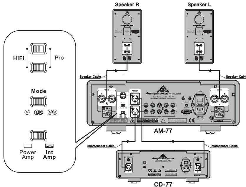
Figure 1.3 - System connection using banana plug/spade connector equipped speaker cables
