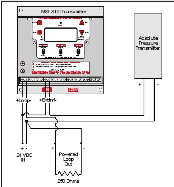
**Four Wire Connection with Absolute Pressure Transmitter**
