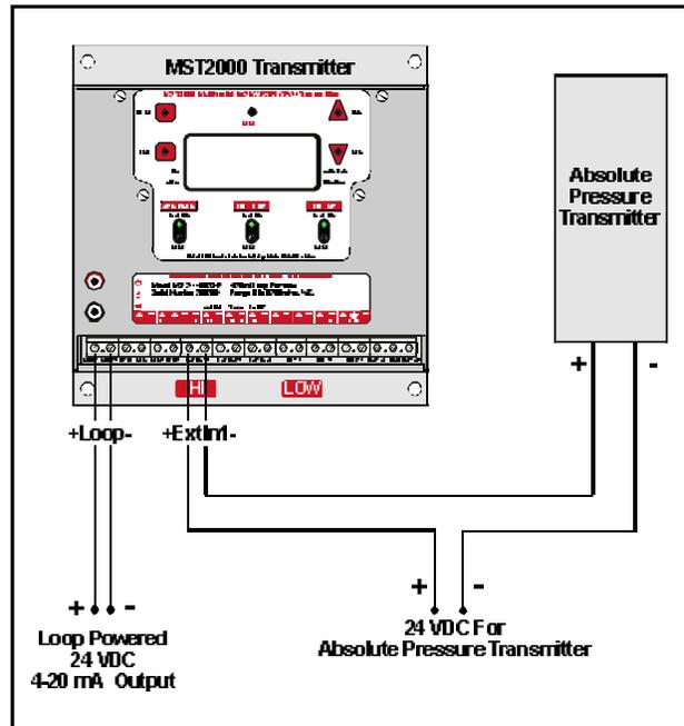
**Dual 2 Wire Connection with Absolute Pressure Transmitter**
