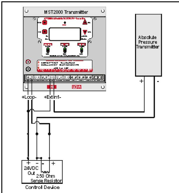
**Three Wire Connection with Absolute Pressure Transmitter.**
