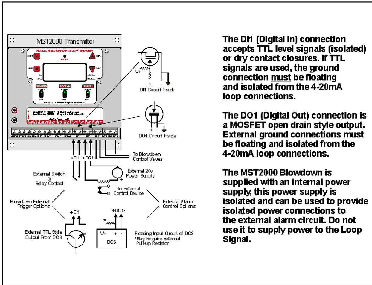
The DI1 (Digital In) connection accepts TTL level signals (isolated) or dry contact closures. If TTL signals are used, the ground connection must be floating and isolated from the 4-20mA loop connections.
