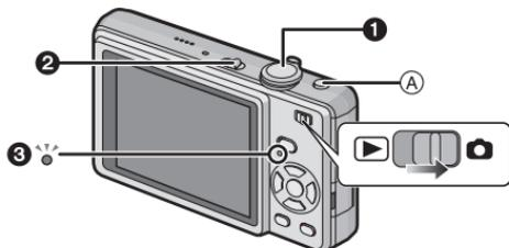
**1** Slide the [REC]/[PLAYBACK] selector switch to **[CAMERA]**, and then press [MODE].
