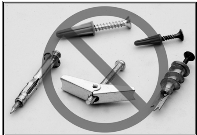
Figure 9. Typical unacceptable fasteners.
