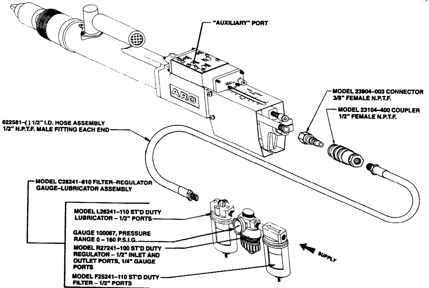
Your ARO self-feed tool is designed to deliver specific horsepower and thrust to achieve high rates of work. To assure the unit will develop this power, care must be taken that the power air inlet system is correctly sized to permit the proper rate of air flow. Shown above is a system for a single tool that will supply correct delivery.
