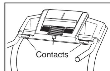
**your heart rate accurately. Before using the handgrip pulse sensor, remove the clear plastic film from the metal contacts. In addition, make sure that your hands are clean.**
