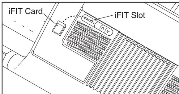
Next, select an iFIT program by pressing the iFIT up and down buttons next to the iFIT slot. When an iFIT program is selected, the display will show the name of the program, the maximum incline setting and the maximum speed setting of the program, and the program time. In addition, a profile of the speed settings of the program will scroll across the matrix.
