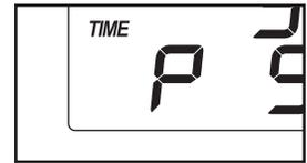
You can adjust the volume of the personal trainer audio (0 through 5) by pressing the 1 Step Incline increase button repeatedly. The volume setting appears as the lower middle digit in the display.
