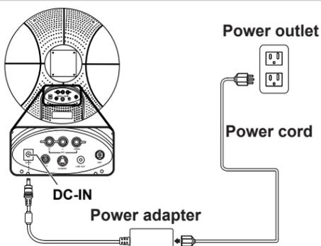
1. Connect the power cord to the power adapter as illustrated.
