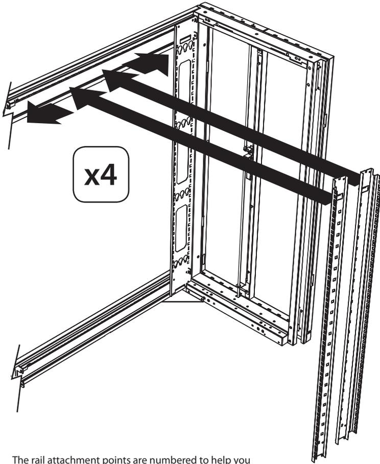
The rail attachment points are numbered to help you align each pair of rails at the same depth. Before attaching the rails using the screws (shown in Step 6-3), make sure the same number appears in all three windows. **Note: Number shown in Step 6-2 is for illustration purposes only; attach rails at desired depth.**
