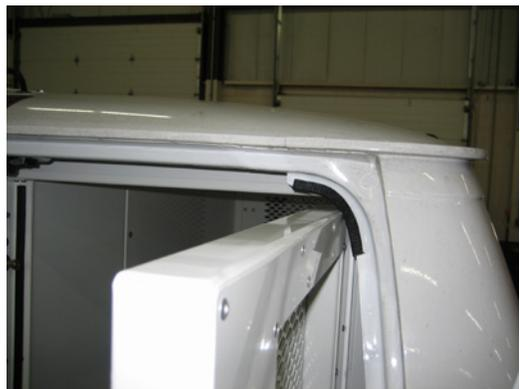
*Note: It is recommended to put edge molding on the OEM door opening on the passenger side to avoid damaging the Kwik kit door.*
