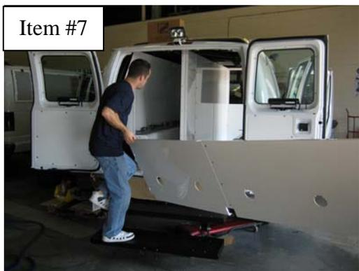
Carefully place **Driver-side Ceiling** section into vehicle.
