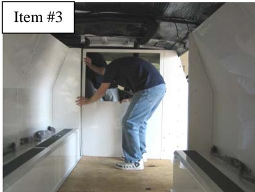
Attach **Front Bulkhead** to **Driver-side Bench/Wall** assembly
