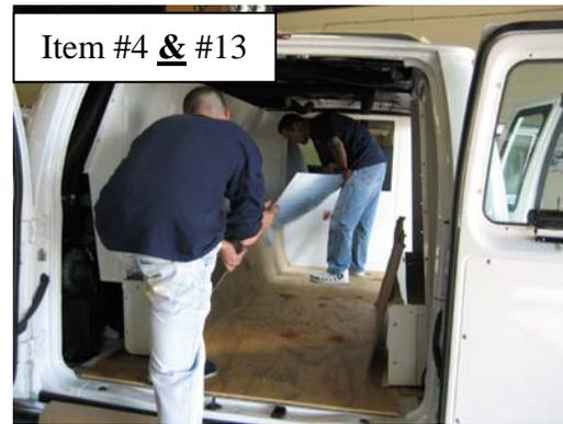
Place (2) **Diamond Plate Floors** between **Bench/Wall** assemblies and **Front bulkhead**. *Place cardboard along side of bench while positioning the floor to avoid scratching the bench.*
