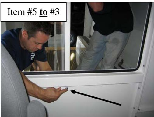
Loosely bolt **Center Divider** to **Front Bulkhead**
