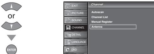
4 Use **[the Number buttons]** or **[CHANNEL - / +]** to select the channel for which you want to check the signal strength.
