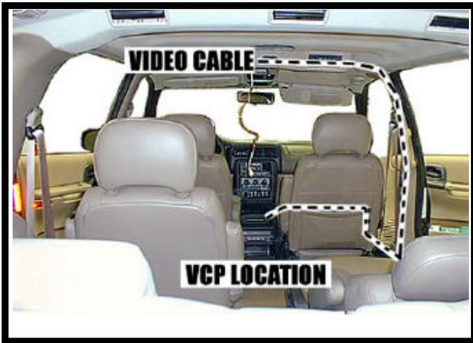
9. Route video and audio cables from overhead console location to passenger's side B pillar. Down B pillar and underneath scuff panel. Up passenger's side kick panel and across the bottom side of dash panel. See Figure 7.
