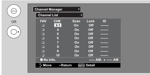
**NOTE:** 1. The Channel List cannot be updated by only changing the cable source. Auto Channel Scan must be performed for the Channel List to be updated.
