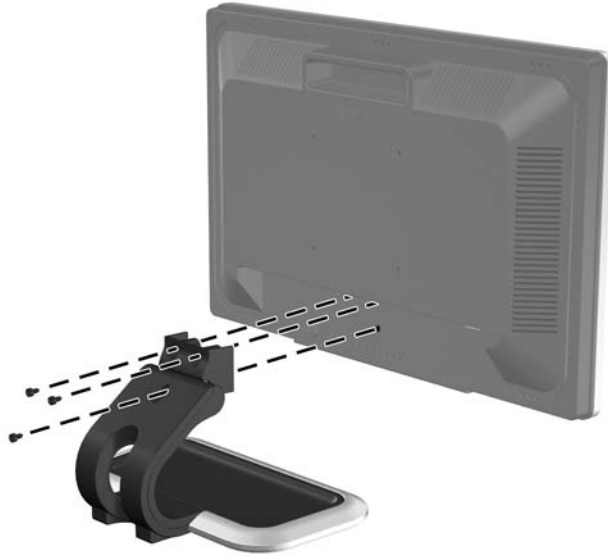
Figure 3-17 Removing the Single-Hinged Pedestal Base
