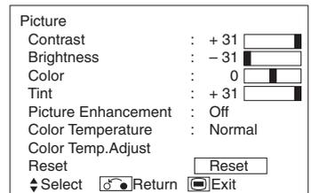
3. Use the ▲ and ▼ SELECT buttons to select the item to be adjusted and then use the ◀ and ▶ ADJUST buttons to adjust (example: Contrast).
