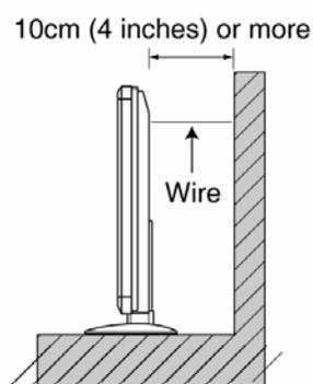
**NOTES:** 1. Do not block the ventilation holes of the Plasma Monitor. Blocking the ventilation holes might cause fire or defect.
