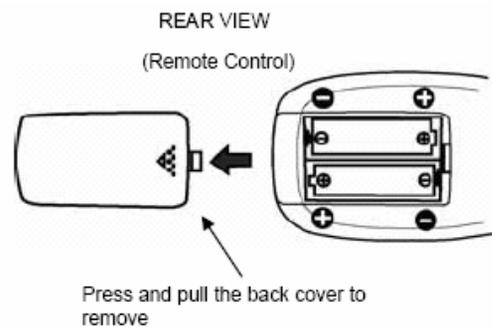
**CAUTION:** Danger of explosion if battery is incorrectly replaced. Replace with the same or equivalent type.
