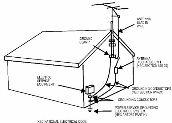
Note to the CATV system installer: This reminder is provided to call the CATV system installer's attention to Article 820-40 of the NEC that provides guidelines for proper grounding and, in particular, specifies that the cable ground shall be connected to the grounding system of the building, as close to the point of cable entry as practical.
