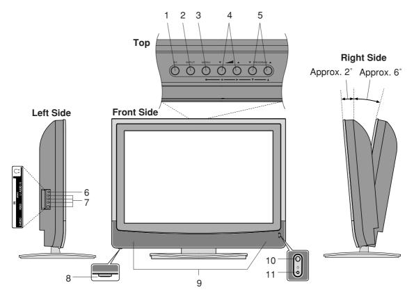
You can adjust the angle of the TV-screen for 2° forward or for 6° backward from vertical angle.
