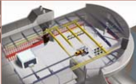
Within the centre, our 850-ton barrier can be positioned and configured to replicate the dangers of countless real-life traffic situations. What's more, this is where collisions take place between a vehicle entering the centre through the fixed tunnel and another entering from a pre-defined angle via the movable test track.
