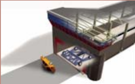
This fixed test tunnel is used for collision tests inside the centre, and for rollover tests outdoors.
